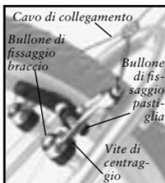
Figure 3.45- Freno a bilanciere o Cantilever
